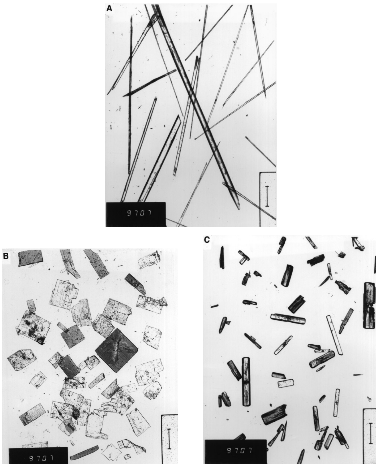
FIG. 1. Optical micrographs of 1 , 2 , and 3 showing crystal habits consistent with the framework dimensionality. (a) Needles of 1-D [\text{enH}_2][\text{Zr}(\text{HPO}_4)_3] up to 1.5 mm in length; (b) plates of 2-D [\text{enH}_2]_{0.5}[\text{Zr}(\text{PO}_4)(\text{HPO}_4)] , typical size 150 \mu\text{m} on edge and 10 \mu\text{m} thick; and (c) rods of 3-D [\text{enH}_2]_{0.5}[\text{Zr}_2(\text{PO}_4)_2(\text{HPO}_4)\text{F}]\cdot\text{H}_2\text{O} ; Scale bar in the photographs is 200, 100, and 200 \mu\text{m} , respectively.
